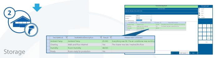
Quality data can also be captured during the storage of raw materials. This test logs the temperature of cold storage units.
