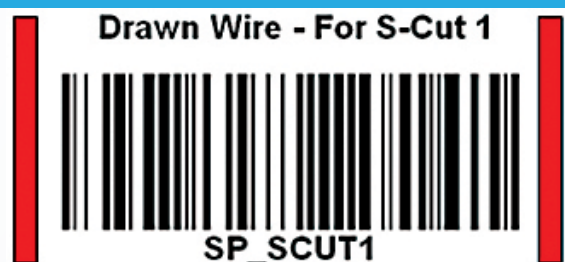
Location label for intermediate product. The location and product labels are all colour coded to allow the operators to easily ensure that the correct product is in the correct location.
